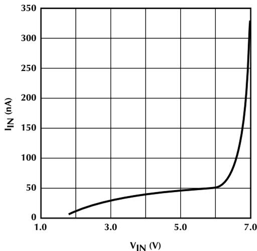
Figure 6. Input Leakage vs.  $V_{IN}$  in Shutdown
