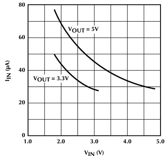
Figure 7. No Load Input Current vs.  $V_{IN}$
