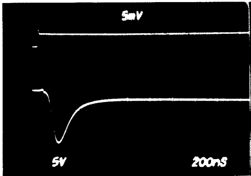
FIGURE 2. Voltage Mode Settling Time—1 LSB Change
